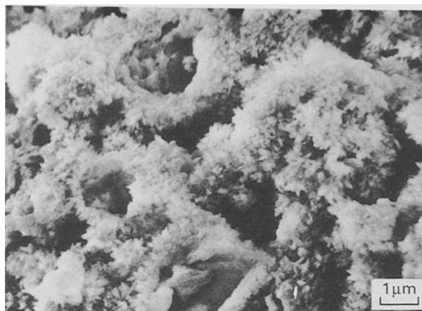
Figure 5 Microstructure of HAp formed in a 150 mM citric acid solution at 38 °C showing the small needle dimensions and hollow shells resulting from citrate adsorption.
